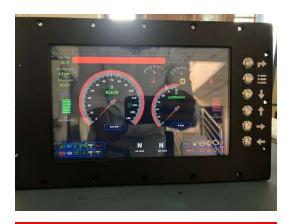
The PRISIM 101 rugged display is a full-featured, configurable display that shows integrated engine data in graphical, alpha numeric forms for easy operator interface. Equipment functionality can be further integrated through the available I/O and controlled via the CAN bus. The RDU101 features a full-color, 10.1"/7 "inch bonded LCD for brighter, smoother graphics and best-inclass sunlight readability. The rugged design makes this display a great solution for extreme environments.
